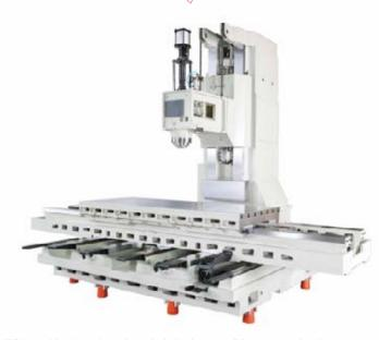
Wide and hardened precise grinded prismatic slide ways on the three axes. Guaranteed stable work by heavy cutting conditions. Super high grade "Turcite-B" fitted to X, Y, Z slide ways.
