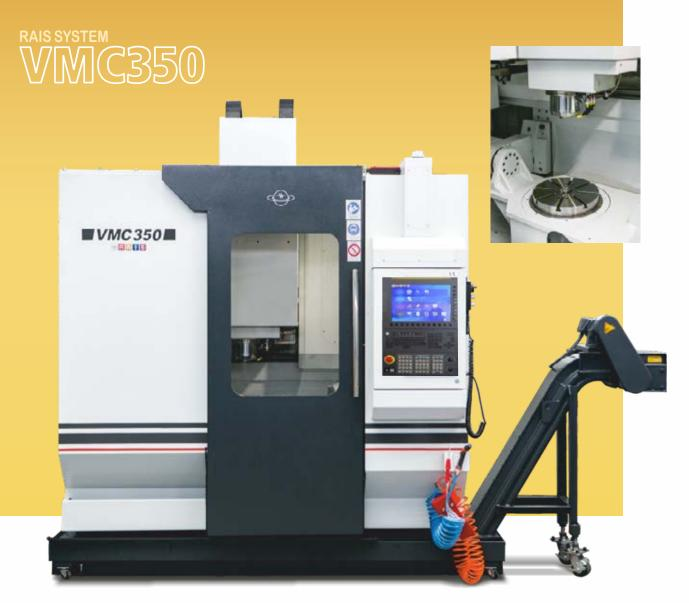
The machine design is distinguished by minimal temperature deformation; absence of vibrations in working process; high and stabile geometry accuracy of finished surfaces.
